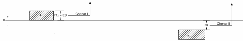
Fig. 1. The values of the tolerance zones in function of the fit type (for clearance fits)
